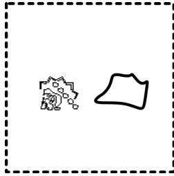
Fig 6a: A reference configuration, captured by an imaging system. We call this “origin image” a “reference frame.” The two arbitrary marks are viewable simultaneously, though they physically reside on separate materials, e.g. a wafer and a mask
