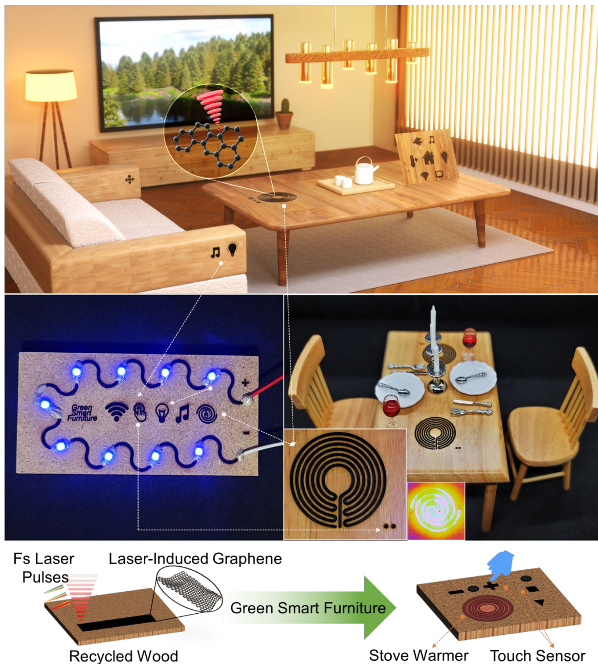
Figure 1. Illustration, modelling sample, and concept image of LIG touch sensor, electric wire for lighting, and stove warmer for green smart furniture applications.
