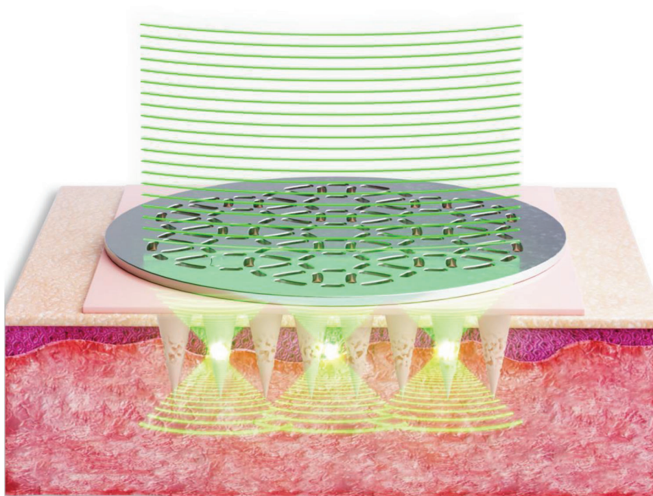
Figure 1. The mobile ultrasound 2D focusing system is based on the dodecagonal quasicrystal patterned (DQP) lens and mobile ultrasound transducer. Planar ultrasound wave propagates through the designed DQP lens and constructs a 2D focal plane at the microneedle. Focusing the ultrasound at the microneedle helps dissolve and activate the drug in the microneedle. This device has been applied in the drug-delivery system.
